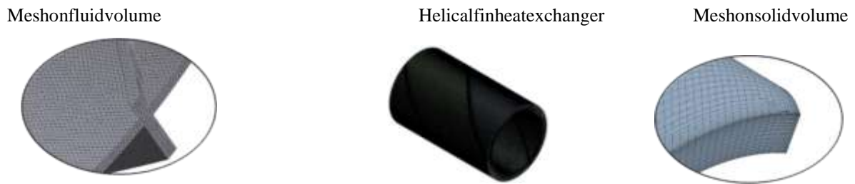
Figure 6: Meshed model of helical fin heat exchanger geometry
